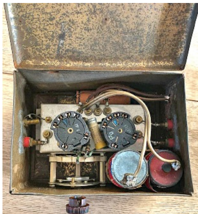
Item #5/2: Internal view of the ostensibly clandestine radio, revealing an apparent German WWII module of unknown origin, two 1.5V batteries, and a rotary switch with a ceramic deck.
