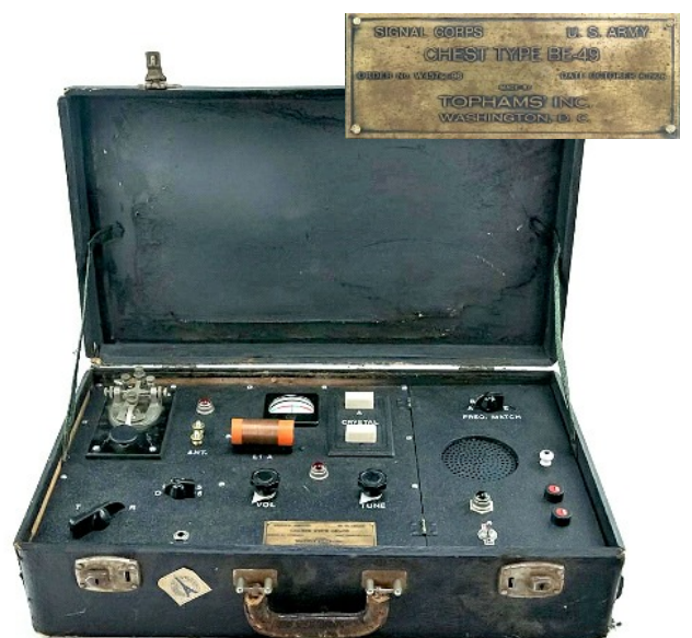
Item #9: Unknown fake / 'replica' set in a suitcase inspired by a Type B Mk.II with a close-up view of the type plate.
