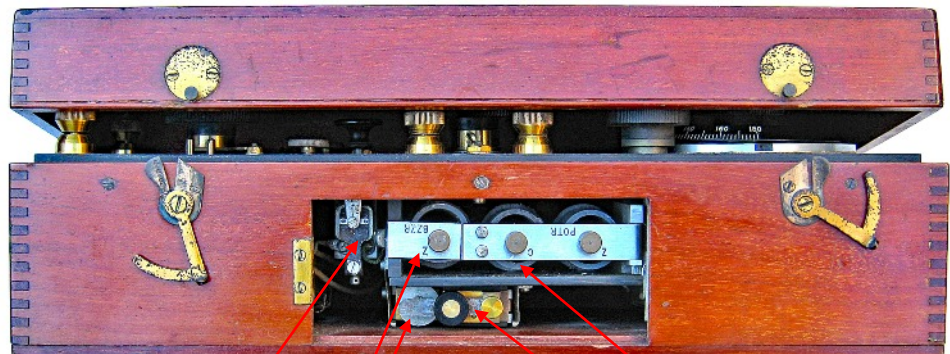
Buzzer The letters 'Z' (zinc) and 'C' (copper) referred to the polarity of the Type E dry cells. Carborundum cup Dry cells for buzzer and potentiometer Detector assembly Detachable panel
