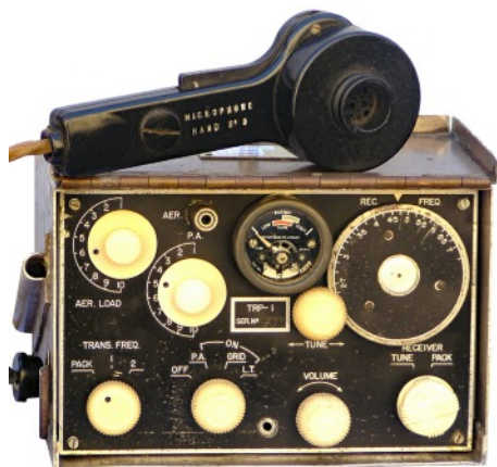
Commercial Pye (Aust) Type TRP-1, a crystal controlled three channel transceiver for AM only (Used 1950-1966).
