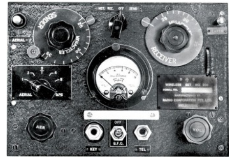
Australian Army Wireless Set No. 208 Mk.I. This set was modified by REC to include AM operation. In use from 1947 to 1958.
