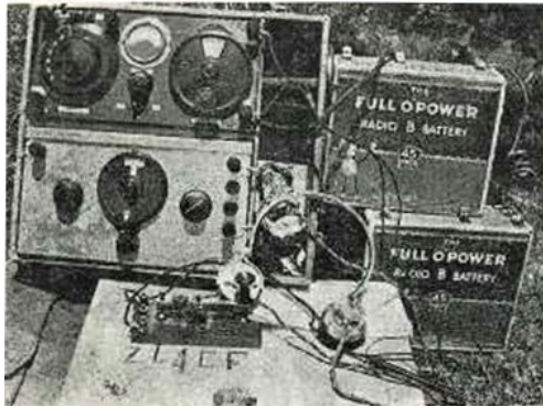
An example of a pre-war portable transmitter-receiver, home made by REC member ZL4CF.
