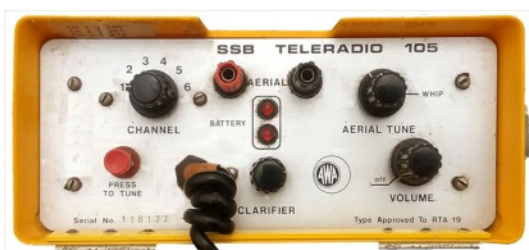
Commercial AWA Teleradio 105: A six channel single-sideband (SSB) transceiver. In use from 1979 to 1990.
