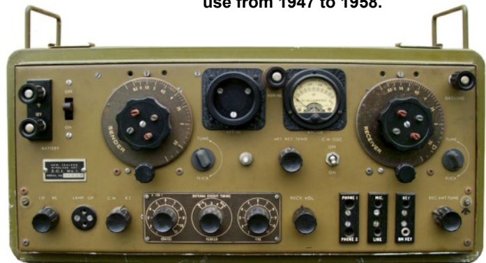
Army Wireless Set NZ ZC1 Mk.I: 60 sets were donated by the War Assets Realisation Board to AREC. They were used from 1949 onwards, operating on AM and CW.
