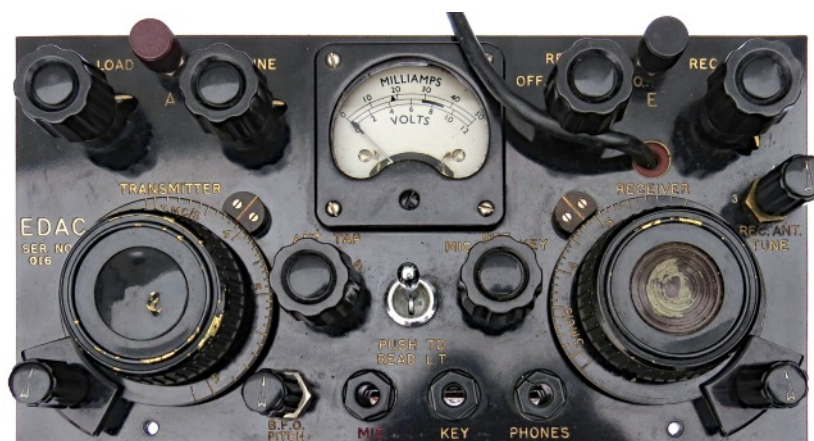
This is an AREC Mark 1 production model (serial no. 016), featuring a simplified meter switch and smaller Philips-type knobs for receive/antenna tuning, pitch adjustment, and dial lock.
