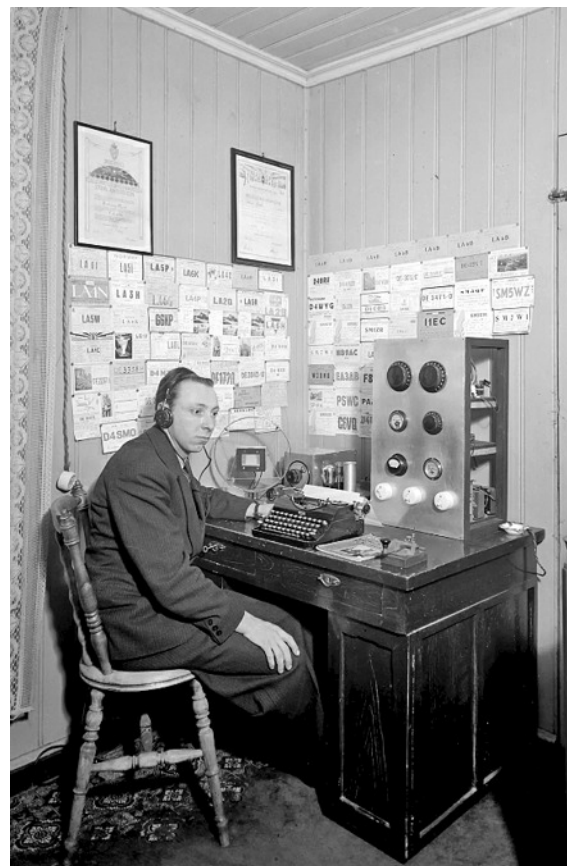
Photographs taken of Gunnar Eriksen, LA6K (left) and Erling Hoel, LA6B (right) at the operating position of their pre-war amateur radio station. Both transmitters (on the table right) shares its construction with the 'Tynset 1940 campaign transmitter' in this chapter and is believed to be an example of a design published in a radio amateur magazine.
