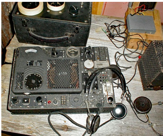
Detail photo of the British Mk.122 from the Stay Behind era. In the background is a Sweetheart Type 33/1 receiver, a 'Svenskesupern' MA 444 and an unknown Morse tape transmitter used with the Mk.122.
