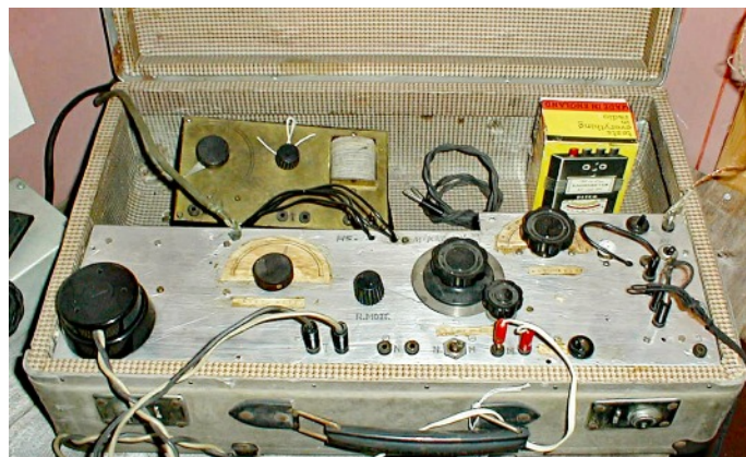
There was no information on the homemade suitcase set, which was most probably constructed after the war. In the suitcase is a Kongshavn receiver.
