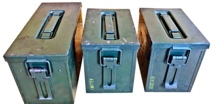
The three units of the set, along with their accessories, were housed into modified ammunition boxes: AC mains power supply left, transmitter centre and receiver right.
