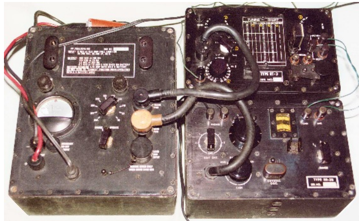
The RS-1 comprised the RP-1 power unit (left), transmitter RT-3 (top right), and receiver RR-2 (below right). It is believed that the RS-5 (RSK-243/SMT-1) was a simplified version of the RS-1.
