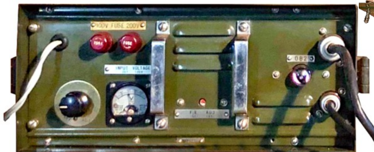
Front panel of AC mains power unit. The top of the 90V receiver OB2 voltage stabiliser protrudes through the front panel, serving as a pilot light.
