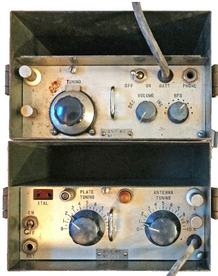
RS-5 (RSK-253) receiver (top) and RS-5 (SMT-1) transmitter (below). Both are low band Type A version, covering 3-7MHz in a single range. Note the modification of the enclosure, a partition created to store the accessories.
