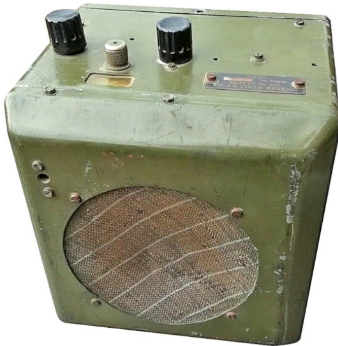
A general view of the Philco BV-613 receiver, which was similar in appearance and internal construction to the BV-611 and BV-612.
