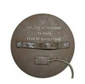
The external pick-up coil known as 'Coil, motor, boat' was permanently fitted in a tug which was used for bridging. It was installed at the rear of the driver's seat, and connected to the Telesonic receiver by a screened cable.
