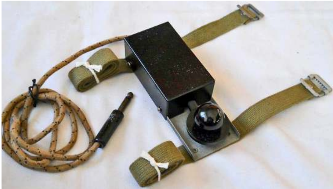
Key and Plug Assembly No. 9 ver. 10.1 was issued with Wireless Set No. 19 Mk.II produced in the USA. This assembly was similar to ver. 10.2. Note the type PL-55 jack plug and low profile protective cover.
