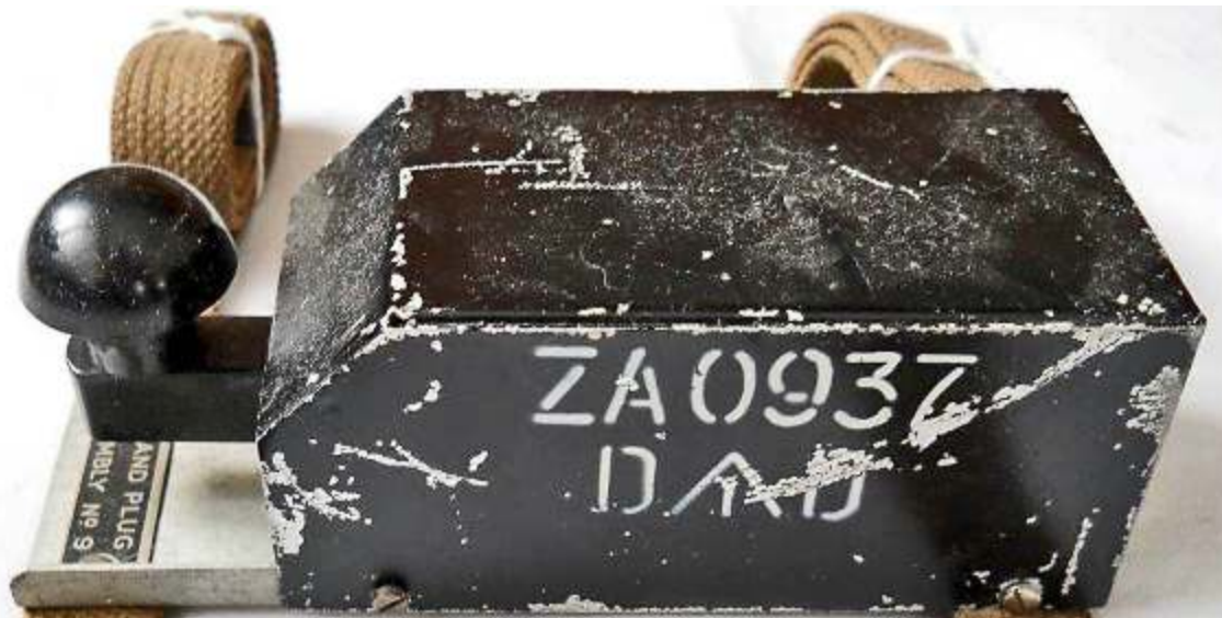
Key and Plug Assembly No. 9 ver. 11 was produced in Australia. This surviving example was fitted with an Australian produced Key W.T. 8 Amp No. 2 Mk.II with three bridges (see below right).
