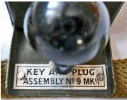
Front view of Key and Plug Assembly No. 9 Mk.1/1 (above) and with protective cover removed (right). Note that all the brass parts of the Key W.T. 8 Amp No. 2 Mk.III and the plug were plated.
