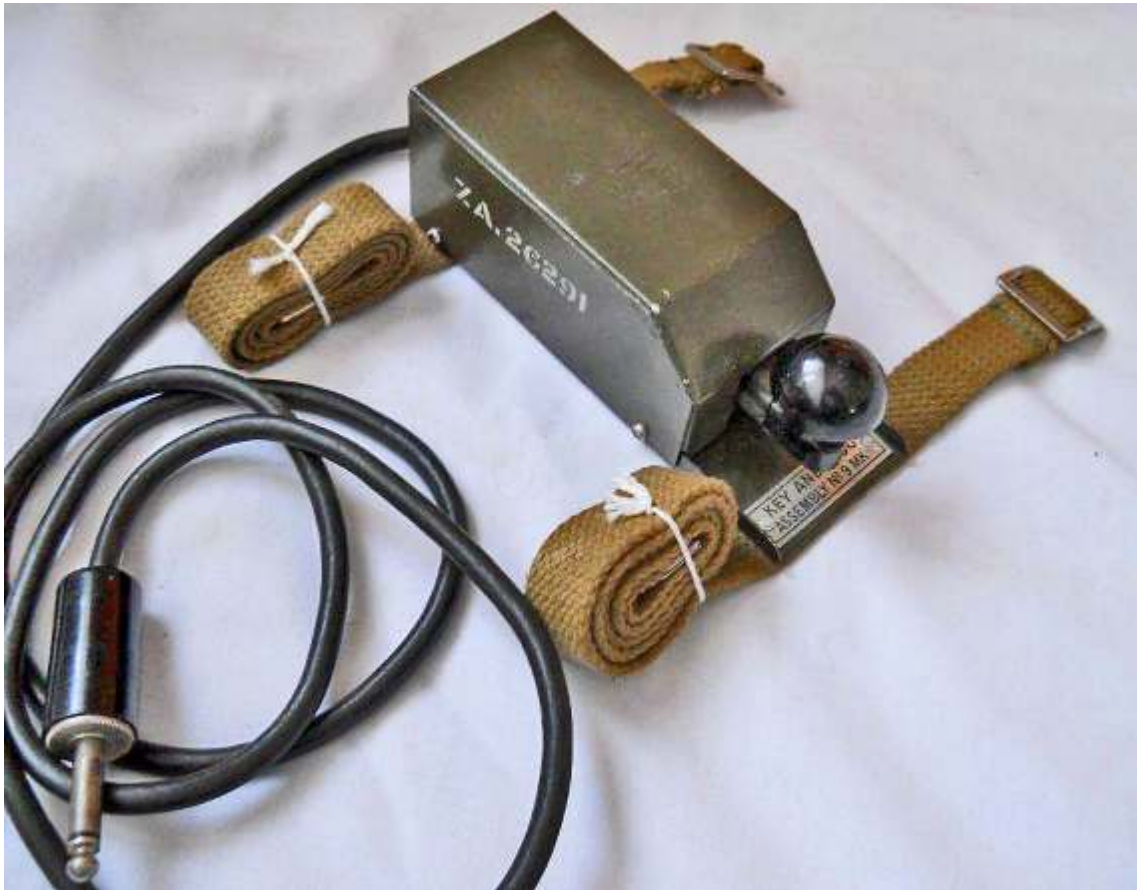
Key and Plug Assembly No. 9 Mk.1/1 ver. 4.3 was the tropicalised version of the No. 9 assembly. It was similar to ver. 4.2 except for having a different type of plug.
