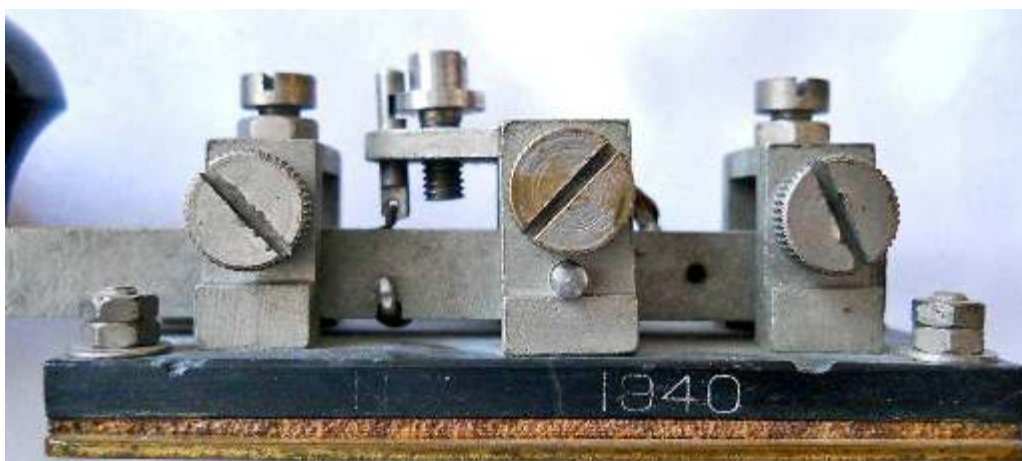
Right hand side view of Canadian Key W.T. 8 Amp No. 2 mounted on a base plate. Engraved on the key base side is the maker's name (Northern Electric Co.) and year of production. Note the Paxolin pad between the key base and base plate.
