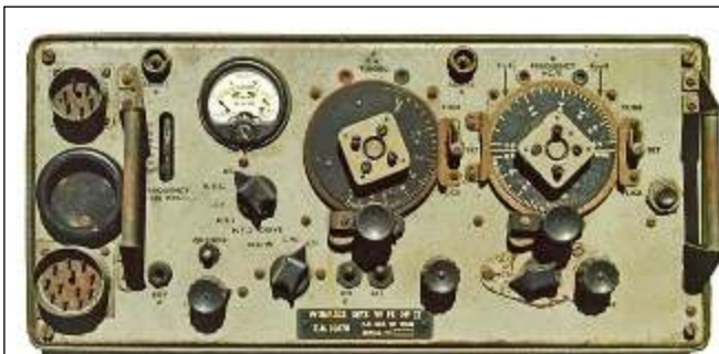
Wireless Set No. 19 (here shown the British Mk.II model, set without power supply unit). Use: primarily developed for AFVs but later used as a general purpose set. Frequency range 'A' set 2-8MHz; 'B' set 229-241MHz. MO control. R/T, MCW, CW. RF output 'A' set 1.2-2.5W (R/T). Range 'A' set up to 15 miles; 'B' set ¾ mile.
