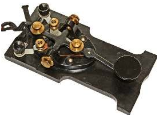
One of the many variations of the American type J-37 key (above).
