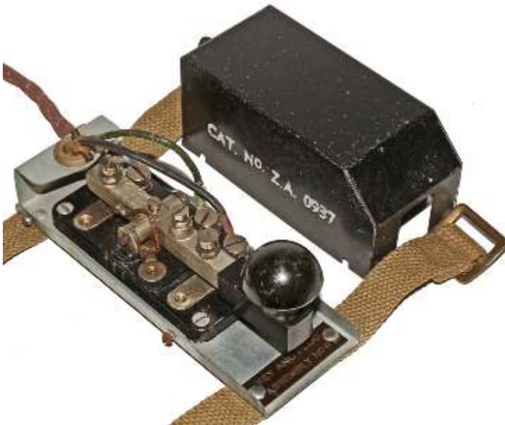
Key and Plug Assembly No. 9 ver. 2 with protective cover opened . The Morse key was a Key W.T. 8 Amp No. 2 Mk.II.
