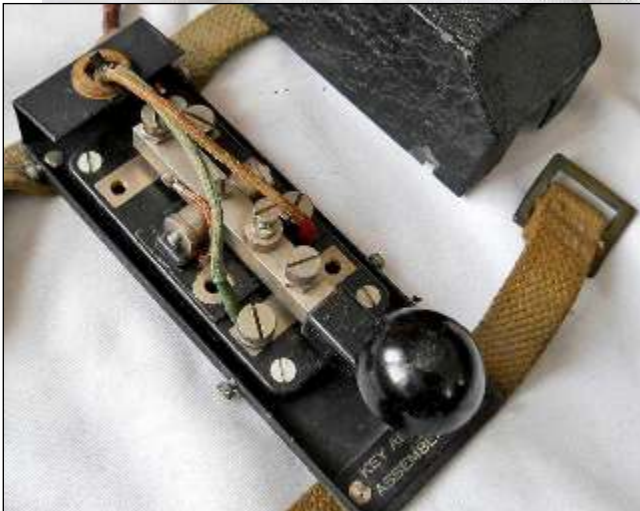
Key and Plug Assembly No. 9 ver. 1 (top of page), and without protective cover (above). The Morse key fitted in the assembly on the picture was a Key W.T. 8 Amp No. 2 Mk.II with a brass key lever.
