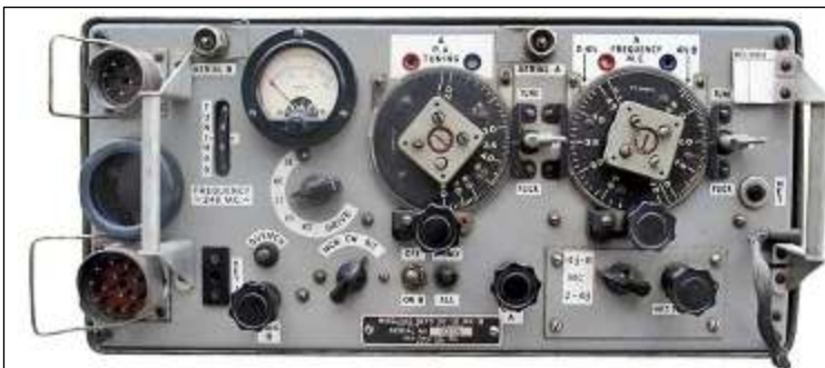
Wireless Set No. 19 Mk.II produced by RCA in the USA. Use: primarily developed for AFVs but later used as a general purpose set. Frequency range 'A' set 2-8MHz; 'B' set 229-241MHz. MO control. R/T, MCW, CW. RF output 'A' set 1.2-2.5W (R/T). Range 'A' set up to 15 miles; 'B' set ¾ mile.
