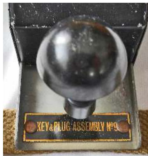
Key and Plug Assembly No. 9 ver. 3.2 with protective cover removed showing a Key W.T. 8 Amp No. 2 Mk.III (left). Detail view of the front with key knob and identification plate (right).
