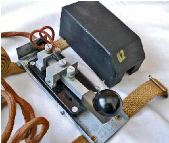
Internal view of Key and Plug Assembly Cdn No. 9 Type 1. Note Key W.T. 8 Amp No. C4 with only two bridges.
