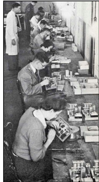
Production of A.E.W. 2 (N.Z.) radios in the HMV plant (right). Note the Staff Sergeant in the background closely observing the workers. An ex-Westco employee who made these recalls that there was an Army inspector on their line checking and, once accepted, broad-arrow stamping each one.
