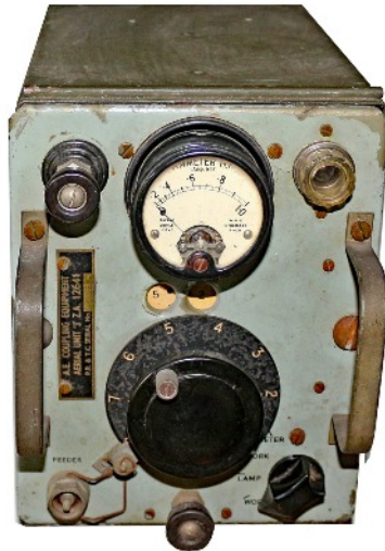
Initial version of Aerial Coupling Equipment, Aerial Unit J, ZA12641. It is interesting to note that this Aerial Unit J came with an Aerial Base No. 10 fitted on top, believed to be a local modification.
