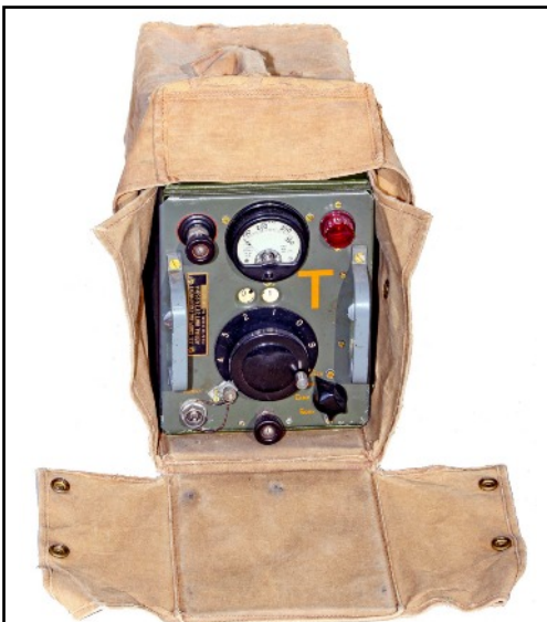
Photograph showing a rare canvas cover for Aerial Coupling Equipment, Aerial Unit JT.
