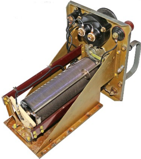
Inside view of tropicalised Aerial Coupling Equipment, Aerial Unit JT, ZA25914.
