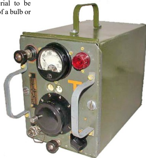
Aerial Coupling Equipment, Aerial Unit JT (above) and circuit diagram (below).
