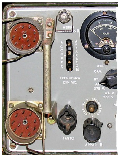
Front panel photo cutout of an Italian Army refurbished Wireless Set No. 19 Mk.III showing the 'B' set section.
