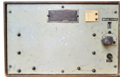
Aerial Tuning Coil No. 2A was electrically similar to the No. 2 Aerial Tuning Coil, but the variable inductor had a different and more accurate counter mechanism.
