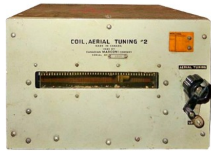
Aerial Tuning Coil No. 2 replaced the Aerial Loading Coil in Canadian Wireless Set No. 9 Mk.I. This unit had a variable inductor with a window showing the position of the slider wheel of the coil.
