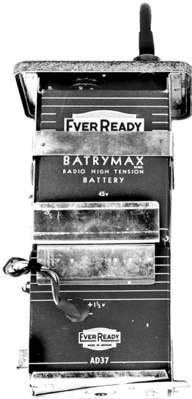
Battery power supply unit comprising two LT and two HT batteries.
