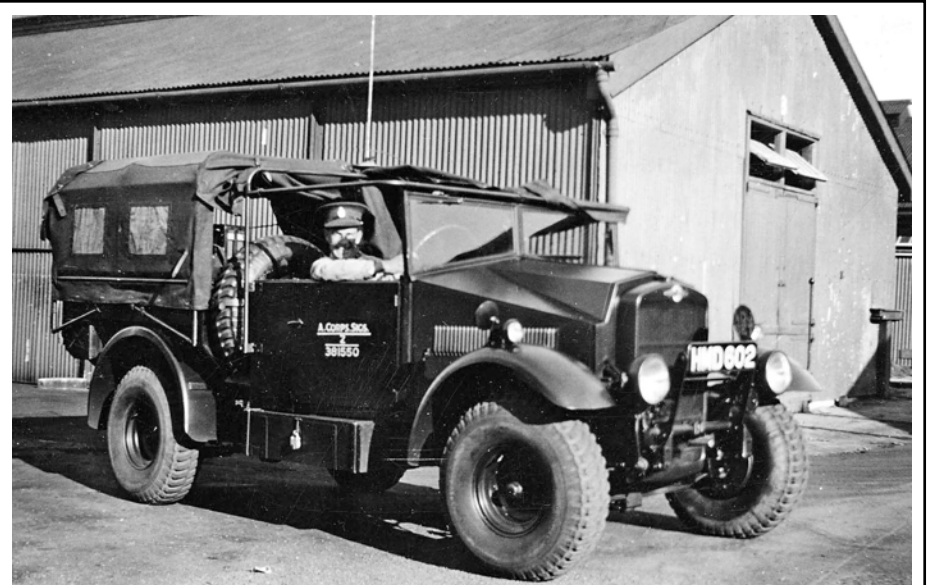
Nouvres, December 1944, at the wheel of a Morris 8-cwt, 4-wheeled wireless 4x2, with 6-cylinder engine, in front of René’s barn. This picture was taken shortly after I acquired the vehicle as a replacement for the wrecked jeep when I rather unwillingly arrived in France. The rather worn-out vehicle was at that time still equipped with a No. 11 Set (mounted on fore and aft off-side shelf) and the old pattern Aerial Base No. 3 and Antennae Rods ‘D’. I had this installation removed as it took too much space for my travels to No. 10 Set locations (Part 2).
