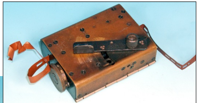
Front view of hand operated tape punch showing punch lever and number setting control. (above)
