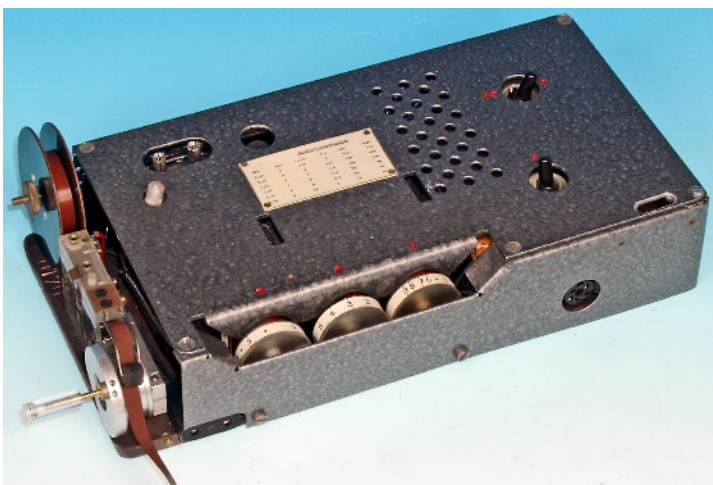
A variation of the Handschnellgeber was permanently attached to a 'Type 2' transmitter with built-in mains power unit. Note a different tape pull mechanism.
