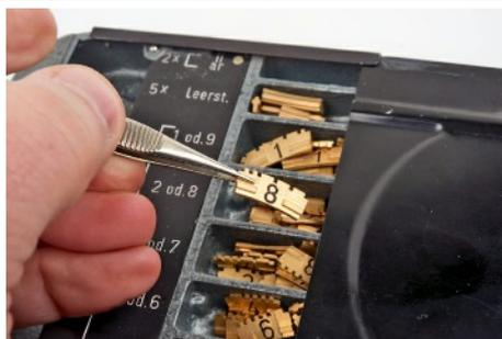
A pair of tweezers was used to pick and place a curved insert into the coder disk.
