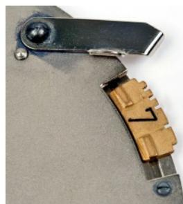
Detail view of loading an insert into the disk which was removed from the KSG Geber during this process. The inserts were placed in reversed order.
