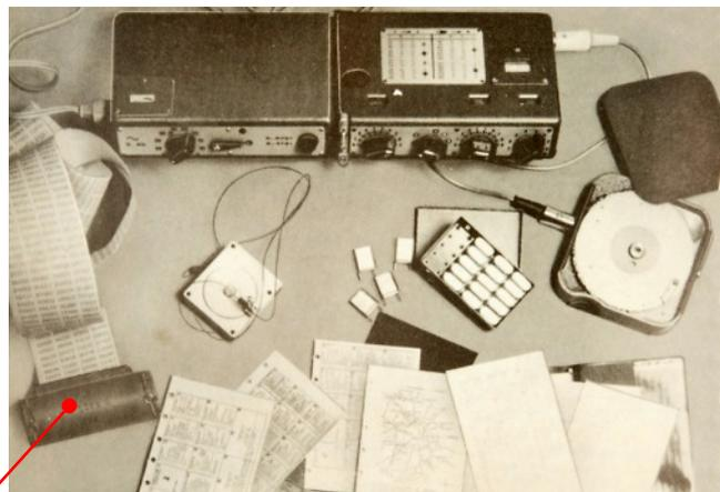
Later version of the KSG Geber here seen connected to a FS-7 transmitter. (Chapter 56)
