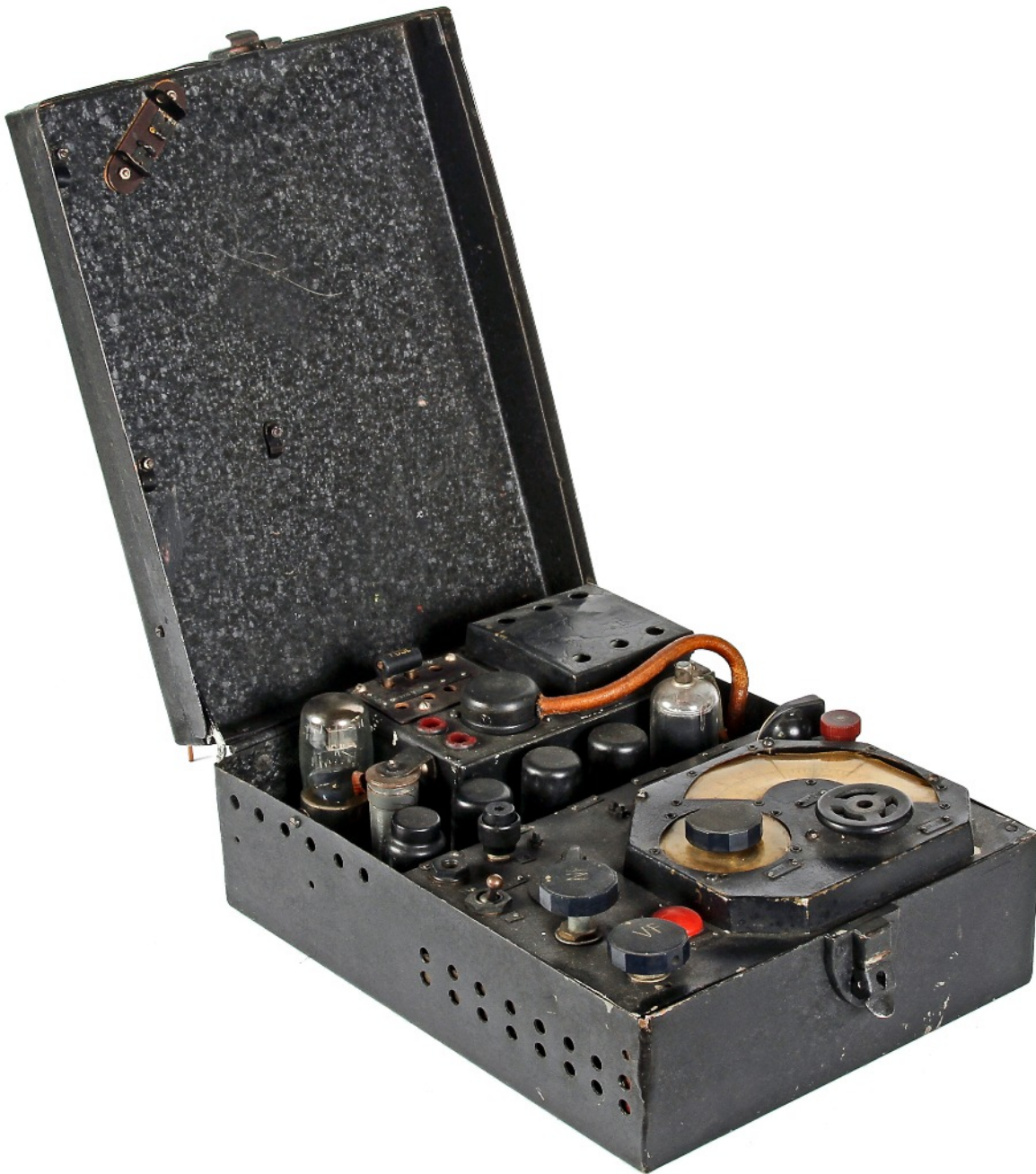
View of a Marjanka receiver kept in the collection of the Military History Institute in Prague. There were minor differences in its construction compared to the receiver on the previous page: no condensers and ballast resistor at the left side in the power unit, and a red control lamp in place of a switch. This appears to be the version of the drawing in WftW Volume 4.
