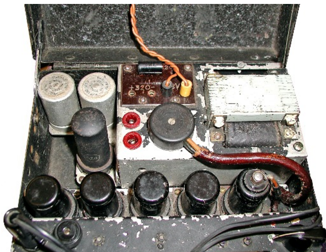
Top view of the Marjánka mains power unit and part of the receiver unit. Note 8-pt plug fitted in the power unit which was also used for connecting the receiver to an alternative LT and HT power source via an adaptor.
