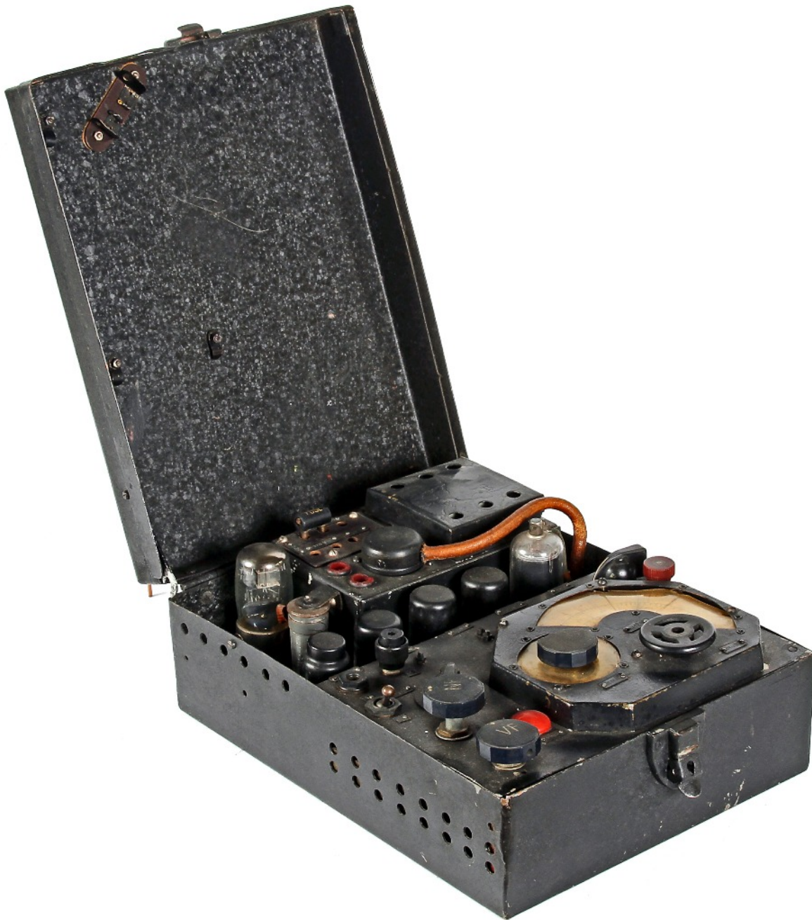
View of a Marjanka receiver kept in the collection of the Military History Institute in Prague. There were minor differences in its construction compared to the receiver on the previous page: no condensers and ballast resistor at the left side in the power unit, and a red control lamp in place of a switch. This appears to be the version of the drawing in WftW Volume 4.
