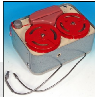
Photograph of a modified Phonotrix ready for recording a Morse code message. (Left) Socket A was for side tone of keying during recording a message and checking in playback or when connected to the receiver listening to the corresponding main station via plug E. Socket B connected the Morse key. Plug C or D connected to the transmitter keying contacts.
