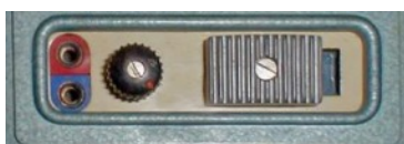
Left hand side panel of the PhonoTrix: Microphone (red) and loudspeaker (blue) sockets (left), playback volume control (centre) and Record/playback switch (right). The two audio sockets were not used in the modified Phonotrix.
