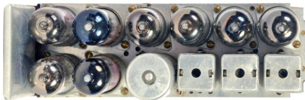
Back view of post war Telefonbogen showing the positions of the valves, IF transformers and BFO coil in a very compact construction.
