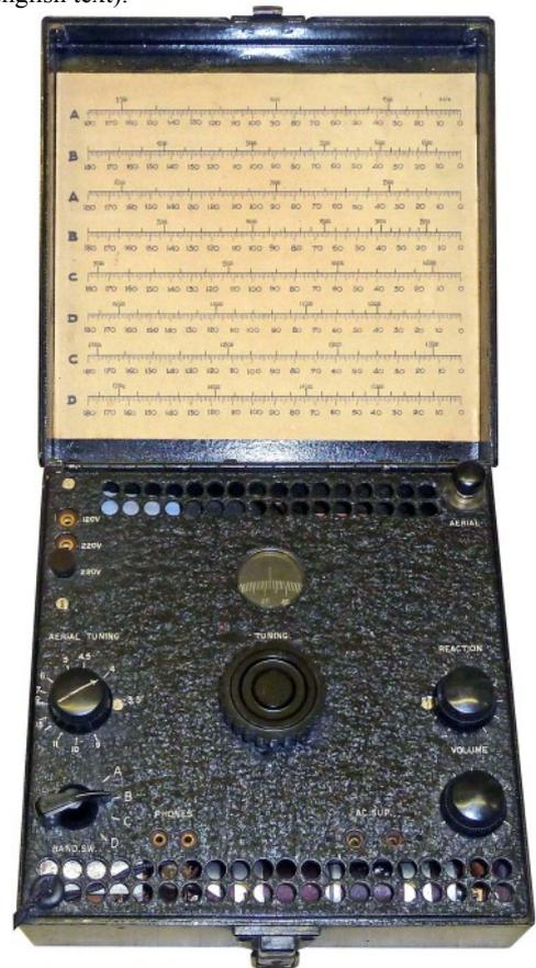
Receiver in metal box with tuning scale calibration card glued to the inside of the lid. The mains lead (bottom left) was fixed and coiled up between the lid and front panel when not in use.
