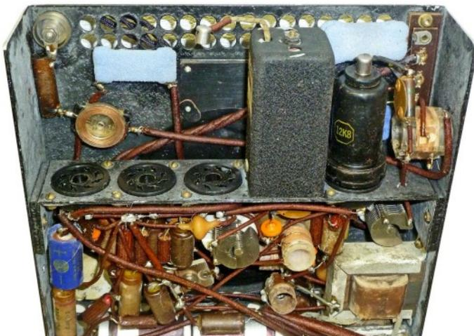
**Top/rear view of the receiver with valves removed showing details of the 1.5MHz IF wave trap and HT ballast resistor. Note the large amount of ventilation openings.**
