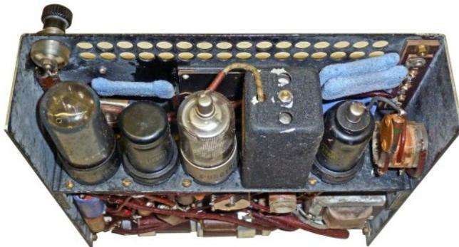
Top view showing the four valves and blue coloured ballast resistors used for the 117N7GT rectifier/AF output valve when used on 220 and 250V AC mains.
