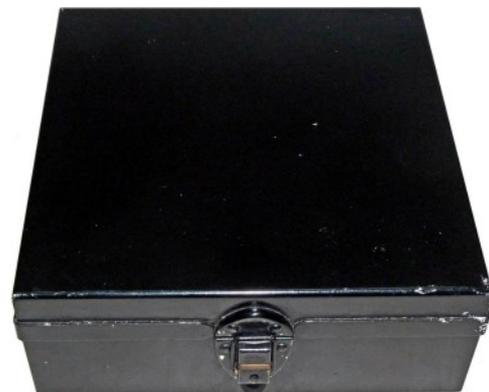
**Enclosure of the Polish 'AC mains SW receiver' with lid closed. This dust proof and water resistant construction was used with most of the Polish sets.**
