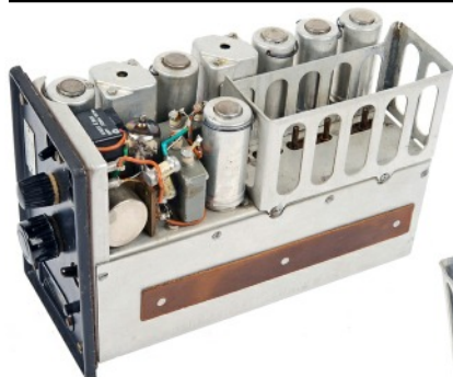
Internal views of the RZ-301 receiver unit. Note the framework which housed the plug-in coil unit. The batteries were carried in compartments located at the rear of the enclosure.
