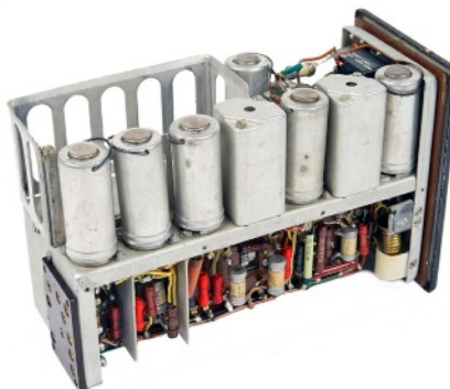
Internal views of the RZ-301 receiver unit. Note the framework which housed the plug-in coil unit. The batteries were carried in compartments located at the rear of the enclosure.
