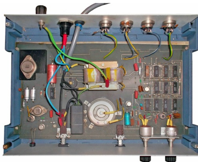
Interior view of AK 1 showing the use of a single circuit board.
