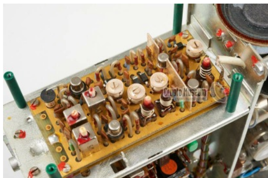
Close up view of circuit board down converter.
