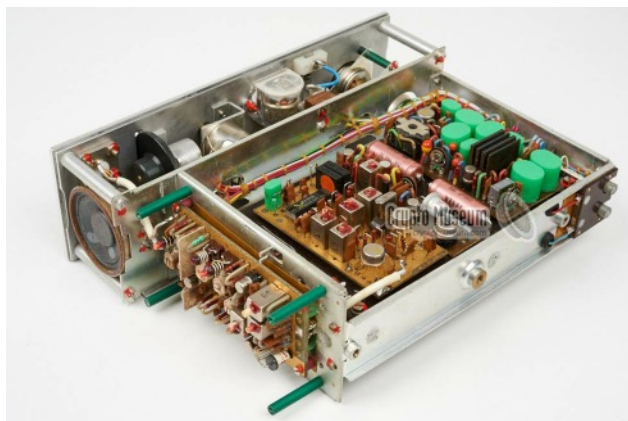
View of chassis Bodrog A. On top are the receiver and AF boards. Located at the side, with its screen cover removed, is the down converter.
