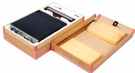
Bodrog receiver with power pack and accessories in transit box.
