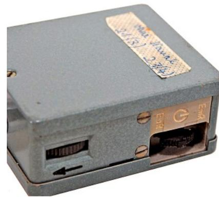
Located on the remote control unit was the volume control, and two control switches positioned at either side of the unit. The transmitter was controlled by a three-position momentary switch (above). The transmitter was off in the centre position. The other two positions were: *SmT* (Senden mit Tonruf - transmission with tone call), and *SoT* (Senden ohne Tonruf - transmission without selective call).
