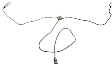
Two different types of aerials were issued with the UFT-421: a rod antenna and a wire antenna (shown above). The latter was an open dipole which could easily be hidden under the operator's clothing.
