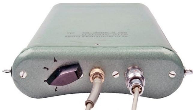
Top panel of the main unit, showing channel selector, microphone/speaker connection and aerial socket.
