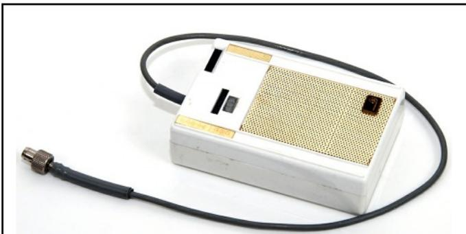
The loudspeaker/microphone of the UFT-421 was disguised as a commercial 'Mikki' medium wave transistor broadcast radio, using only the enclosure. These radios were commonly used in the GDR at the time and would not attract much attention to the public. It allowed the operator to hang around, pretending to be listening to a broadcast transmission, whilst in reality receiving instructions or passing status information.
