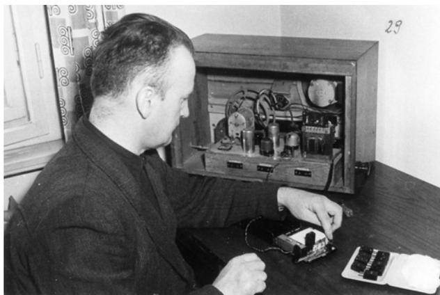
Photograph taken by the former GDR MfS of a 'Camera' transmitter as it might have been used by an agent. Note a box with spare crystals for operation on alternative frequencies.
