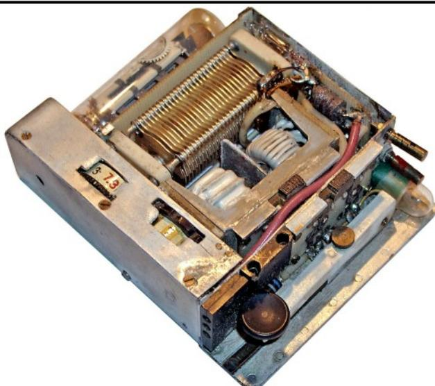
Side view of the 'Camera' transmitter with outer cover removed showing from left to right: tuning condenser, aerial matching switch, two aerial coils, range switches and crystal socket. Visible just behind the Morse key was a bulb for tuning the aerial by max brilliancy. On the side in front was a 3-point socket for connecting a special cable leading to an EL84 valve socket. The Morse key could slide forward when in operational use.
