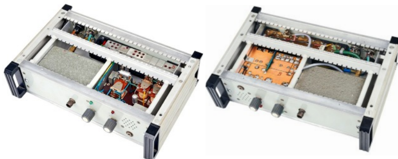
Top view (left) and bottom view (right) showing the fully enclosed down converter, control board and receiver unit.
