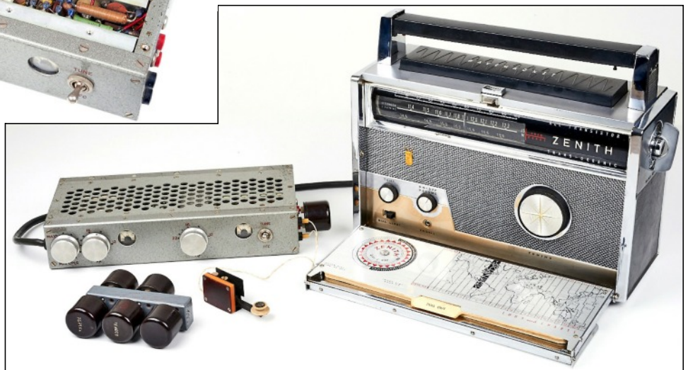
'Kongo' station with transmitter, associated Zenith receiver, hand speed Morse key and crystals. The external matching power unit is unfortunately missing.
