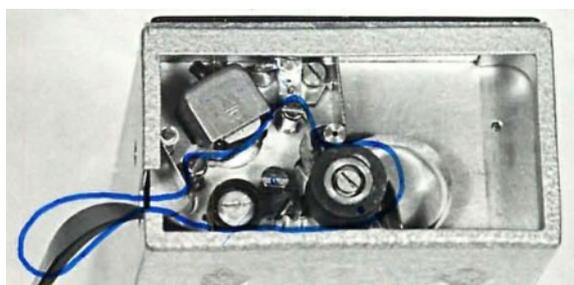
Endless tape record/playback assembly of Dávač (above) and Mesic (below).
