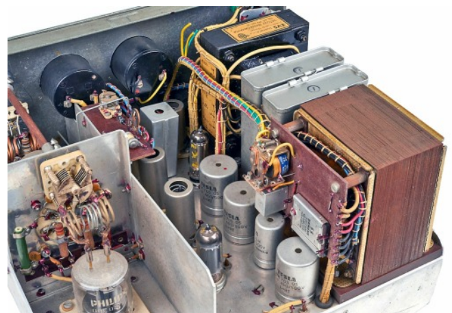
Top view of 'Davor' showing mains power unit at the right; the MO, modulator and driver stages centre. The tripler and RF output stage to the left. (above)
