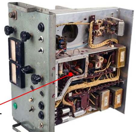
Top view of 'Davor' showing mains power unit at the right; the MO, modulator and driver stages centre. The tripler and RF output stage to the left. (above)
