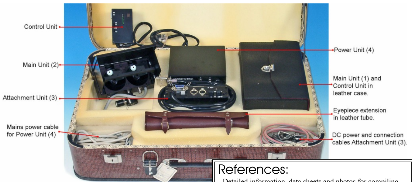
Transit suitcase for a pair of sets with 2x JO-4.03 (Main Unit (1) right and Main Unit (2) left), Control Unit, Attachment Unit (3), Power Unit (4), cables and eyepiece extension.
