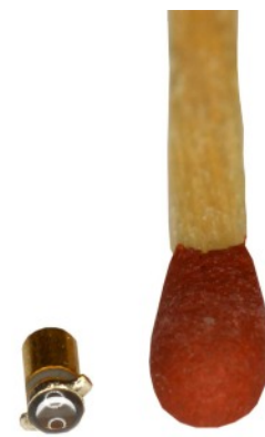
Size of an infrared led compared to a match.
