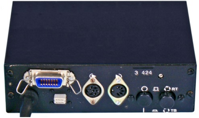
The Attachment Unit (3) was used for automatic operation of a JO-4.02 or JO-4.03 Main Unit (2) in combination with a tape recorder. The unit was connected to the Main Unit in place of the Control Unit, which in turn was connected to the socket top left.
