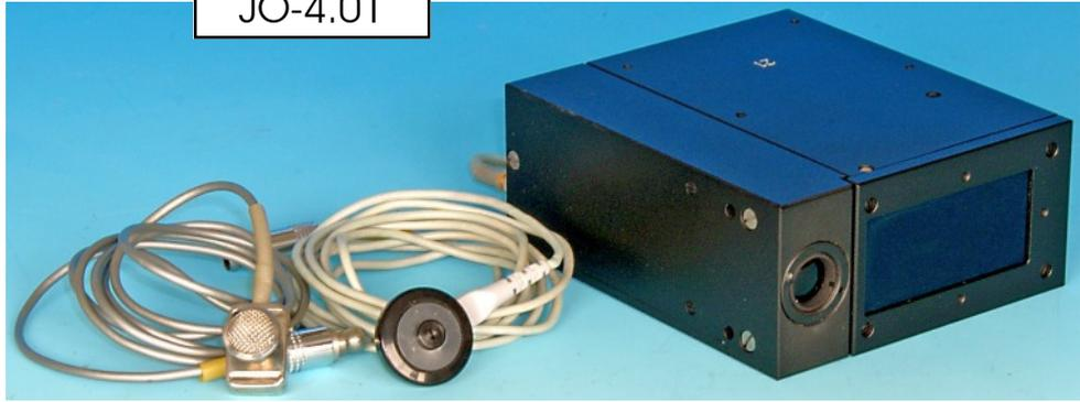
JO-4.01 was a passive infrared set with a range of about 500m. It was the successor of the 'Rostock' and operated in combination with a JO-4.02 or JO-4.03 at the other side of a link. Though originally used for transmitting in one direction only, optionally a separate receiver unit (left) could be bolted to the left hand side allowing two way conversation, primarily for use by agents.
