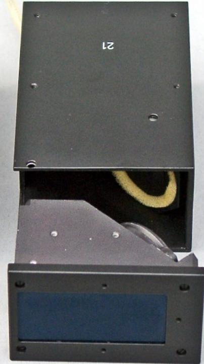
View of disassembled main assemblies of a JO-4.01.
