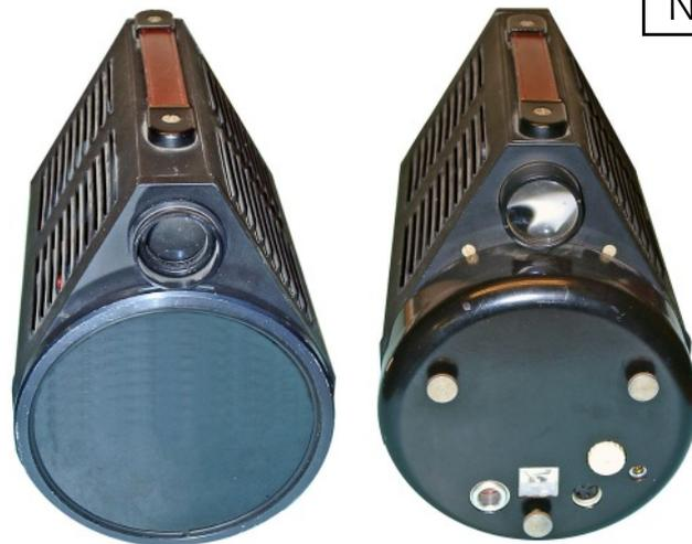
'Neiße' was used in combination with the 'Rostock' passive infrared set. Seen from front (left) and rear (right). It radiated an unmodulated infrared beam and received the modulated reflected beam.
