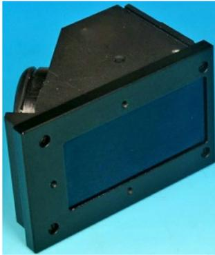
Mirror and diaphragm assembly of the JO-4.01. When placed behind a window pane it could transmit conversations in that room.
