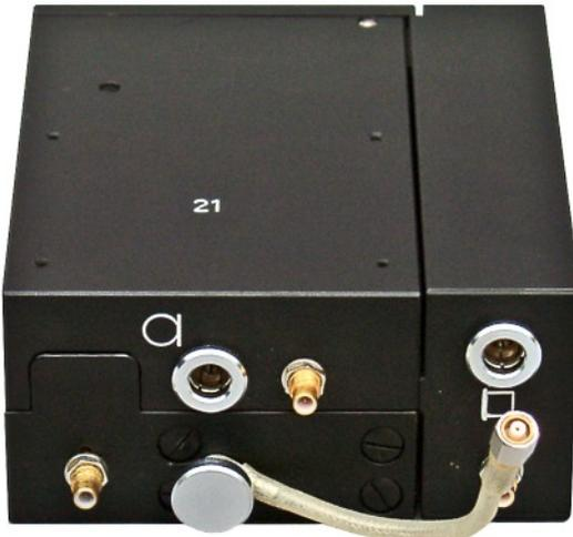
Rear view of JO-4.01 (left) and separate receiver unit (right).
