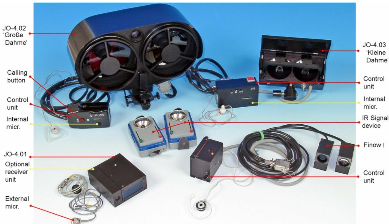
Overview of currently known infrared communication equipment developed in the GDR. Top left: JO-4.02 known as 'Große Dahme'; top right: JO-4.03 'Kleine Dahme'; bottom left JO-4.01, a passive IR set; bottom right Finow I; in the centre infrared signalling devices disguised as ordinary electric torches. (See Chapter 69).
