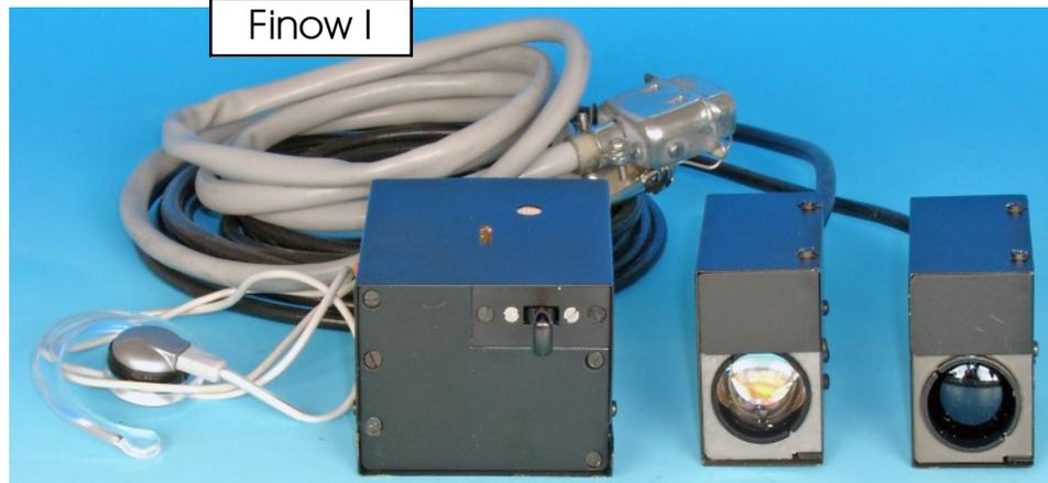
Finow I comprised two separate main units: The transmitter (left) and receiver (right with dark lens) which could be bolted together or used separately, both connected to the Control Unit in the centre-left side of the photo.
