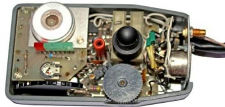
Internal view of control unit with cover removed. Note the microphone (top left), black calling button and volume control below.
