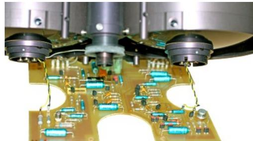
Internal view of JO-4.02 as seen from the rear. Conventional components and transistors were mounted on the PCB. The set had an integrated battery compartment for three AA alkaline batteries. The later developed JO-4.03 was designed with mainly ICs manufactured in the GDR.
