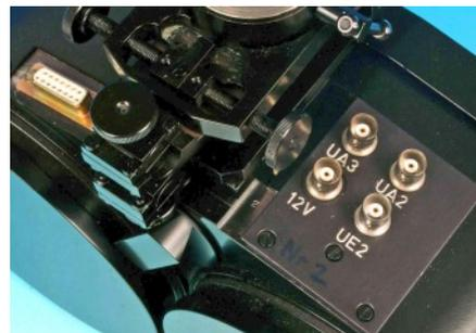
A modified JO-4.02 used for one way transmission of video was known as JO-4.05; at the opposite side was the JO-4.06. The external differences to the parent model were extra BNC sockets and a different type of system socket at the bottom.
