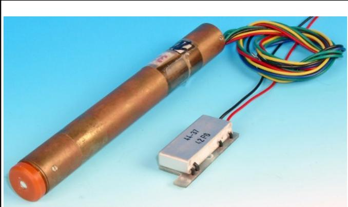
Infrared bug for transmission of conversations picked up by a hidden microphone. The other side of the link could be a JO-4.02, JO-4.03 or even a Finow I of which only the receive side was used.
