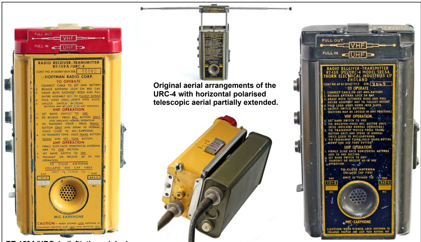
The mercury battery pack (right) had a twistlock arrangement which fastened it to the back of a URC-4.
