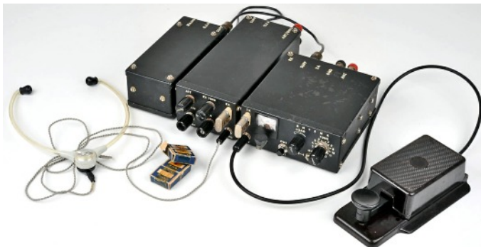
Complete RTP8-SSB/3 station (AC power supply left, receiver centre and transmitter right) with an often used German WW2 Junker Morse key.
