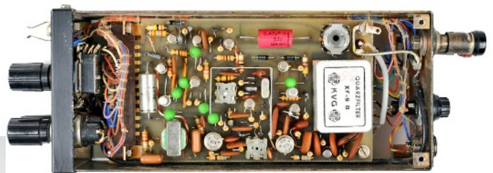
Bottom view of receiver unit showing the IF board with 9MHz crystal filter, IF, detector, BFO and AF stages.
