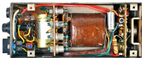
Internal view of the AC mains power supply.
