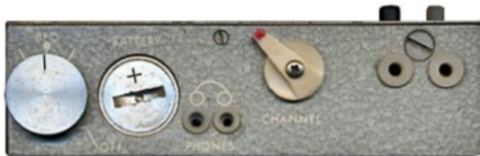
Side view of RR-48A showing from left to right: BFO adjustment control, battery cap, earphone sockets, channel switch and earth/aerial sockets.
