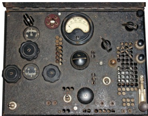
Front panel view of an original Polish BP 4 with receiver section fitted. See also Chapter 47.
