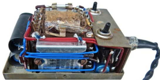
Internal view of 'Type 1' AC mains power supply unit.
