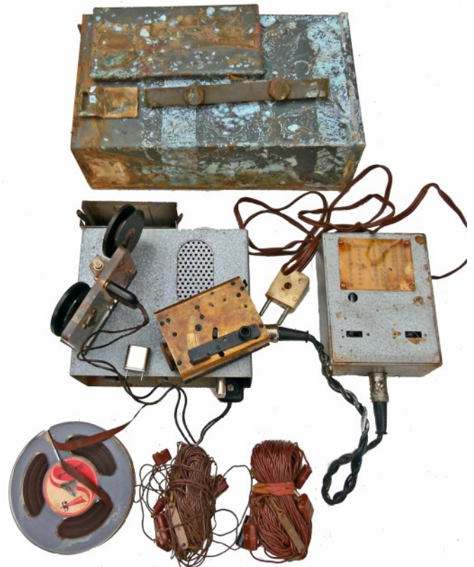
Metal container and complete 'Type 1' set which was found buried near Paderborn in Germany. One of the metal retaining clip plates of the container had been rusted away by which a minimum amount of moisture could enter.
