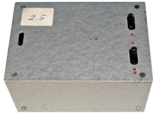
AC mains power unit issued with a 'Type 2' transmitter. Variations in construction of this unit are noted.
