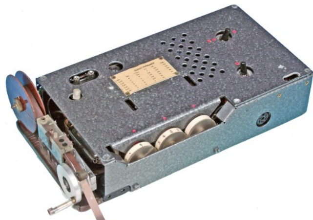
Transmitter 'Type 4' was essentially a 'Type 2' with built-in AC mains power unit (right hand side with two switches) and a Handschnellgeber (See Chapter 98) fitted at the other side of the set.
