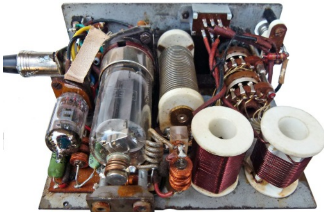
Internal view of the buried 'Type 1' transmitter. The crystal oscillator valve was a Russian type 6x1n, a near equivalent of a 6AK5 valve which was fitted in another surviving 'Type 1'.
