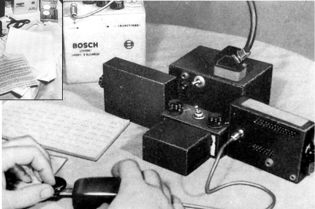
'Modular' set as it might have been used by agents, powered by a 6V accumulator. Note the use of a German World War 2 'Mouse' Morse key.
