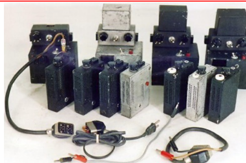
Four 'Modular' sets. Note cables in front for connecting the power unit to AC mains (centre) and 6V DC (left - right).
