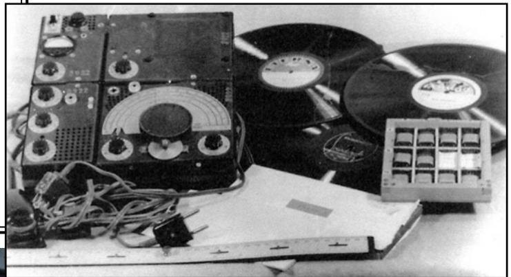
12WG four-unit variation set captured in possession of an agent in the GDR. (Above). Along with the 12WG came a box with crystals for operating on other frequencies, code tables and a set of 78rpm records with a Morse code course. The 12WG was complicated and mainly issued to agents with a background in operating similar equipment, for example former military signallers.
