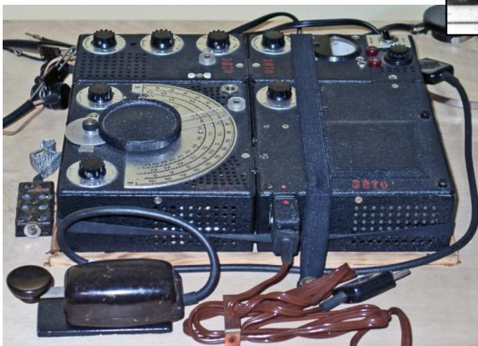
A 12WG with accessories as kept in the DHM (Left). Note the use of a WW2 'mouse' Morse key and transmitter aerial dummy load left in front of the receiver.
