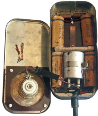
BP 5 microphone. Internal view of opened microphone.
