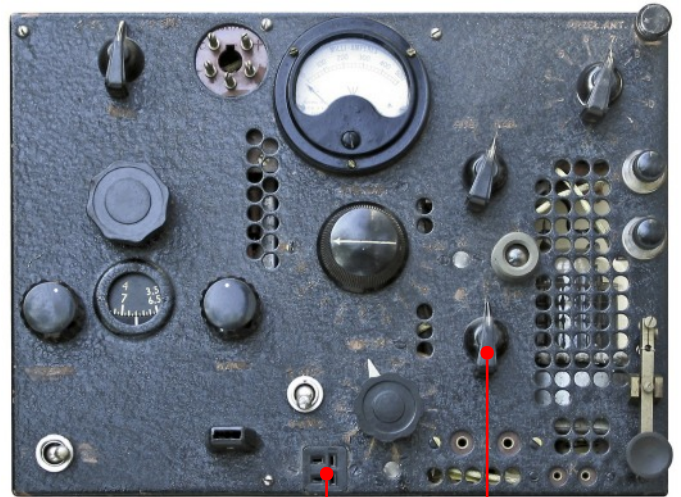
Polish BP 5 showing the 4-pt microphone socket (1) and 3 position switch (2) replacing a tumbler switch. The set was otherwise nearly identical to the BP 3.
