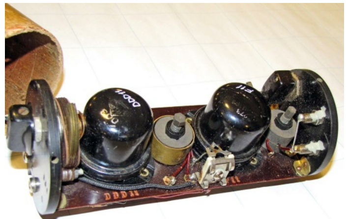
Top view of opened Töpö: from left to right: reaction control, DDD11 double triode metal valve (detector and AF stage), detector coil in dust iron core, pre-set trimmer detector coil, DF11 metal valve (RF stage), and aerial coil.
