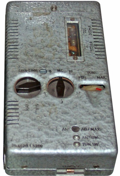
Transmitter unit (3-12MHz) with mains power supply.
