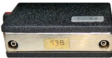
Side view of plug-in unit showing the contacts to the main unit. (left). The units came in two different sizes: - Units 1, 2, 7, 8, 9 and 10 were small in width (1.8cm) - Units 3, 4, 5 and 6 were larger with a width of 3.9cm.
