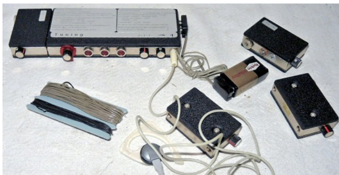
General view of the FLE receiver fitted with a plug-in unit and three additional units for other ranges. The 9V battery could also be plugged in directly to the side of the receiver.
