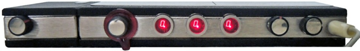
Front panel view of the FLE receiver showing (from left to right): Plug-in unit RF amplifier tuning; main tuning control with fine tuning; 7 segment led displays; system switch: AM - display on - CW; volume control; earphone socket.
