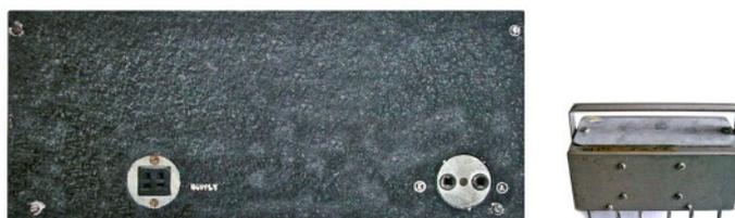
Rear view of cabinet and Plug-in coil box (up to scale). The receiver had a separate battery box connected to the 4-point socket at the left.
