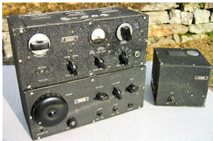
General view of Mk.26 receiver (below) and Mk.25 transmitter on top. The vibrator power unit shown at the right was for the Mk.25 transmitter only. The Mk.26 receiver had miniature battery valves and was powered separately from dry batteries.
