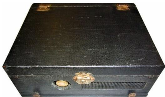
General view of French 33X 'suitcase' set with front lid closed. Note the round opening with push button which was used as an emergency Morse key.
