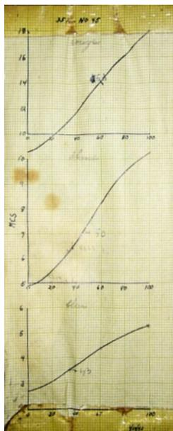
Frequency calibration graphs of the receiver tuning dial, attached in the inside of the lid.
