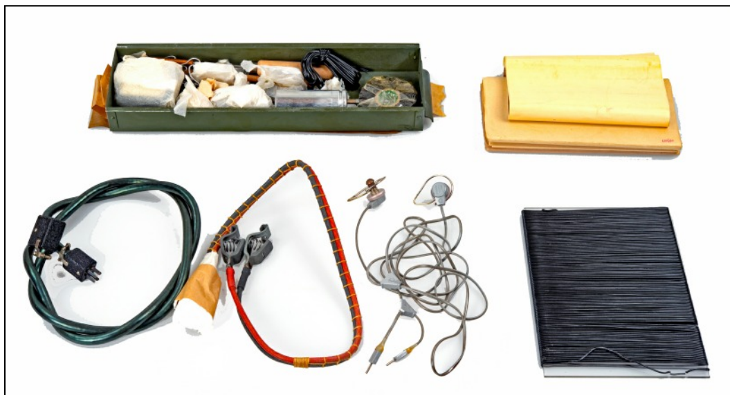
Mk. 122 accessories and spare parts in a tray. Considering the 6V battery cable, a four-pin connector and spare vibrator, a Supply Unit Vibratory No. 14 was issued with the stay behind station.
