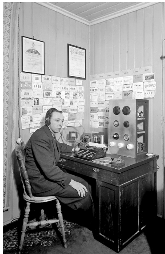
Photographs taken of Otto Eriksen (left, call sign unknown) and Erling Hoel LA6B (right) at their operating position of their pre-war amateur radio station. The transmitter (on the table right) shares its construction with the 'Tynset 1940 campaign transmitter' in this chapter and is believed to be an example of a design published in a radio amateur magazine.
